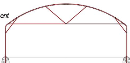
tension rods reinforcement
